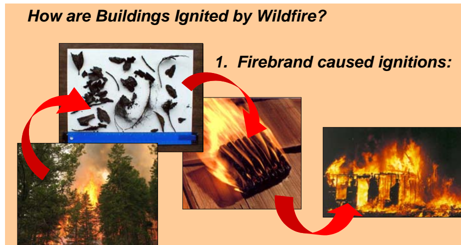
Figure 4. Firebrand caused ignitions: burning embers are carried ahead of the fire front and alight on vulnerable building surfaces.
