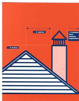
Figure 11. Standards for chimney design as per Fire Smart: Protecting your Community from Wildfire.
